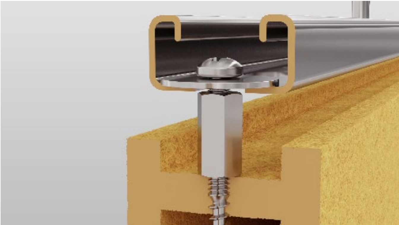
Direct mount to Unistrut with Bolt (male), Coupler, Washer, and Screw
